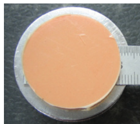
xantasil shrinkage behaviour after several weeks.
