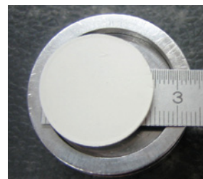
Shrinkage behaviour of leading competitor alginate after 24 hours.
